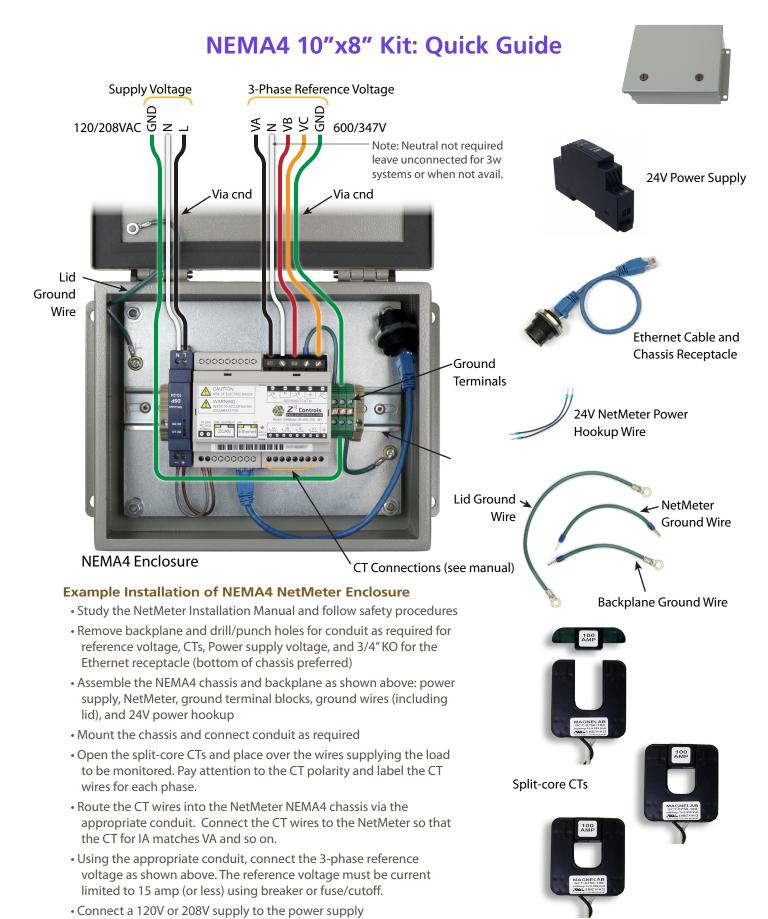
Mount the Ethernet chassis receptacle into the 3/4" hole
