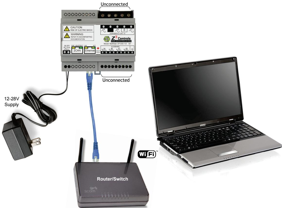
**Figure 9: NetMeter Setup Used to Perform Initial Configuration**
